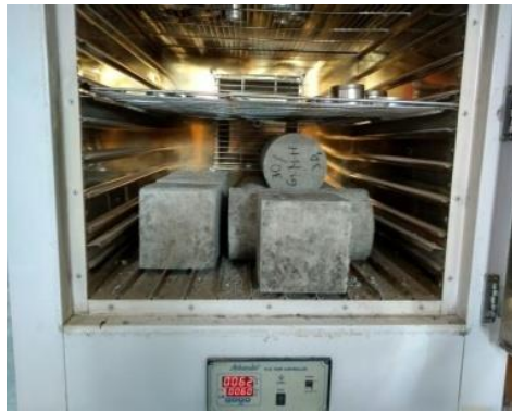
Fig.8. Oven curing of Geopolymer-Concrete specimens
