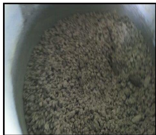
Fig.7. Fresh Geopolymer Concrete mix
