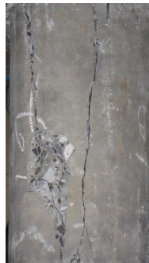
Fig. 9 Nucleation of inclined fracture surface and diagonal fracture zone
