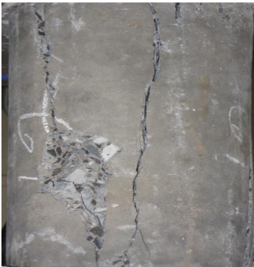
Fig. 5 Inclined fracture surface and diagonal fracture zone for cylinder
