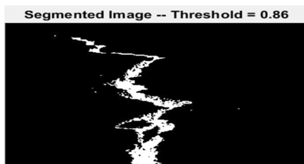
Figure 5 Segmented of longitudinal crack image and thresholding
