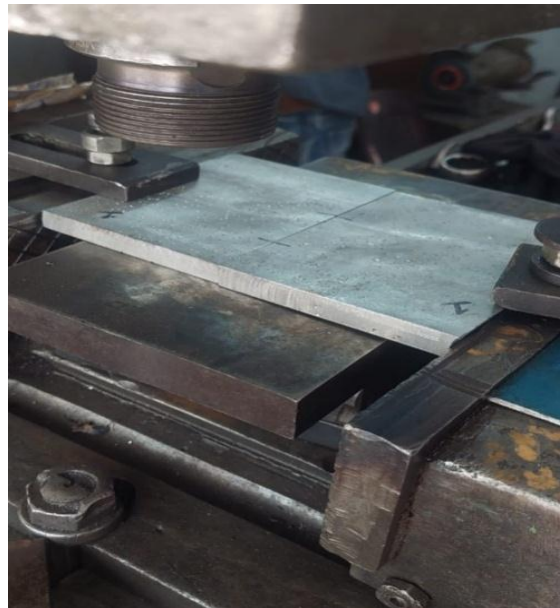
Fig2 FSW process using vertical milling machin
