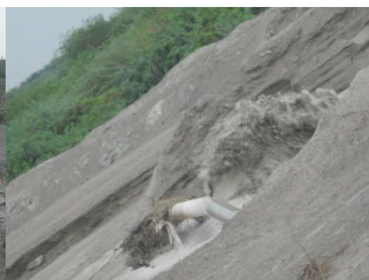
Figure 1(b) Ash transportation by pipe
