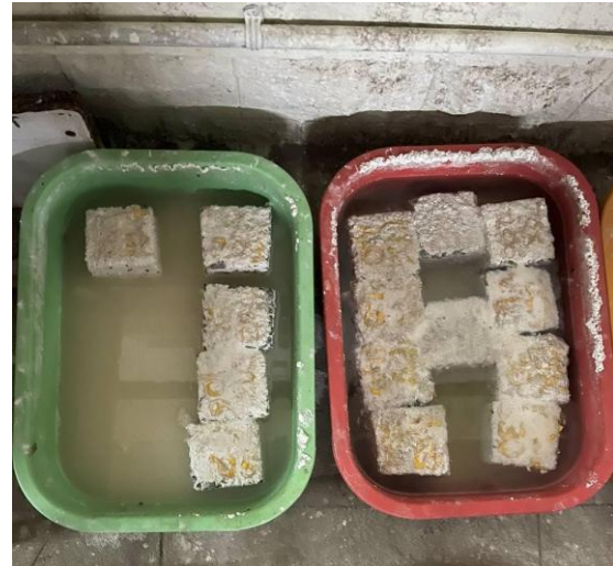
Fig 6-Curing of specimen in acid solution
