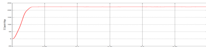
Figure 8: Simulation Results for DC capacitor voltage.
