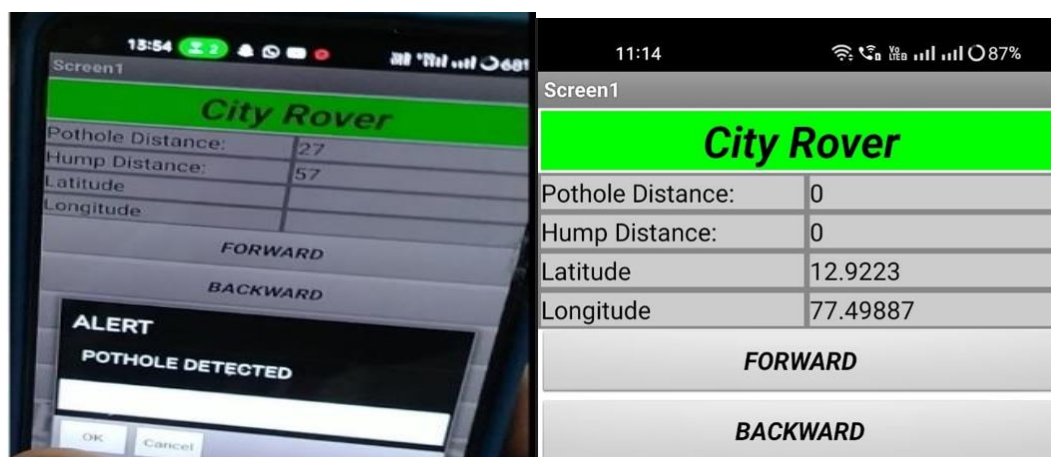
Fig.2.1.2. Pothole alert displayed on the mobile phone.
