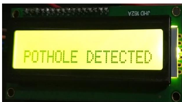
Fig.2.1.4 Pothole alert displayed on the LCD Display
