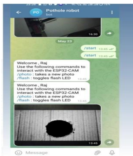
Fig.2.1.5 Pothole image captured by ESP32 cam..
