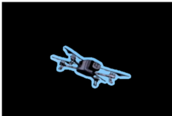
Figure 4. Segmentation of objects using the MoG (Mixture of Gaussians) method (background has black color).
