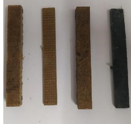
Fig 4(b) Tensile test samples of (coir, hair, jute + coir and jute +Glass) composites.
