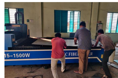
(c) Plate placement in CNC
