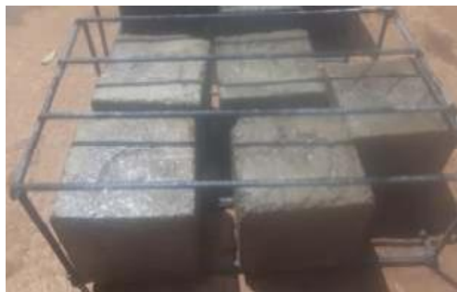
Figure 3: Concrete Cubes Suspended on a Steel Frame, Ready for Immersion in Acidic Solution.
