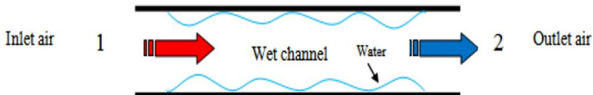
a) Working principle of direct evaporative cooling
