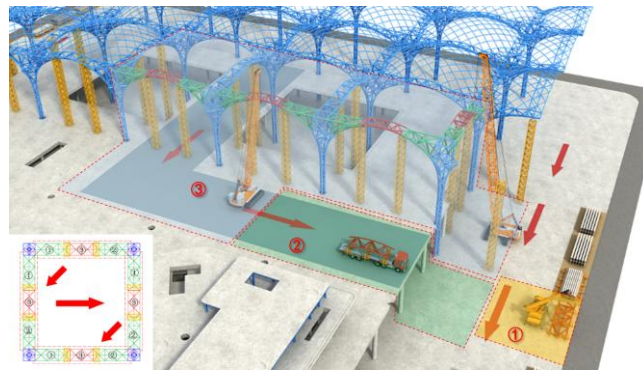
Fig 21 Virtual construction drawing for truss lifting
