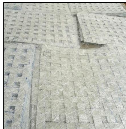
Figure 1. Alternating Fiberglass Placement in Each Layer
