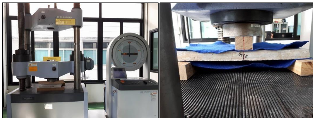
Figure 6. The Tile Breaking Strength Test
