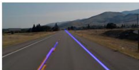
Fig 10: Image showing edges after Hough transformation
