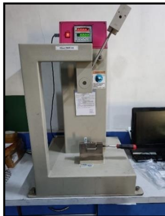
Figure 5: Impact test specimens during the test
