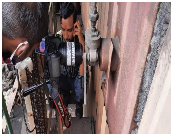
Fig 3:- Real time data acquisition of Flame Images
