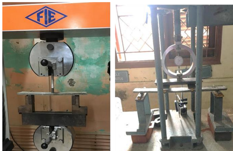
Figure 5 Test set-up; (a) three point flexure, (b) four point flexure.
