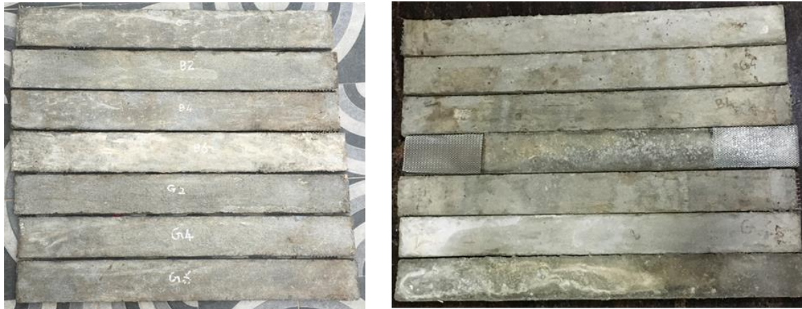
Figure 4. TRM Flexure specimen.
