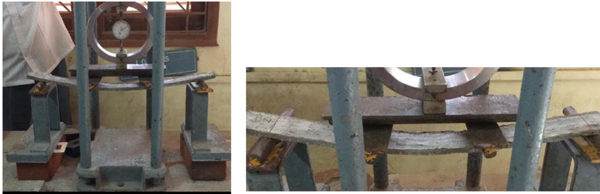
Figure 9. Four point flexure test failure specimens.
