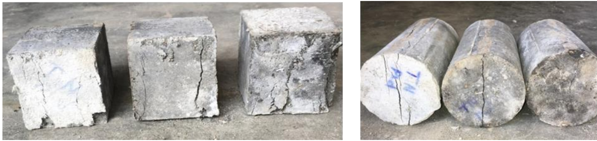
Figure 1 Failure of (a) mortar cubes, (b) mortar cylinder.
