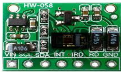
Fig. 2. sensor module of MAX30102.
