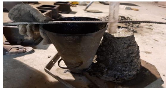
Fig. 4 Slump cone Test
