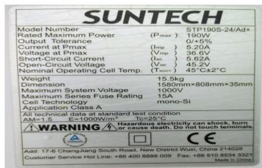
Fig.3. The photovoltaic module nameplate of our system
