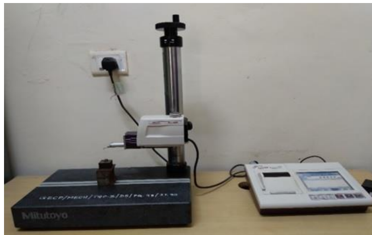
Fig. 1. Surface roughness measurement apparatus
