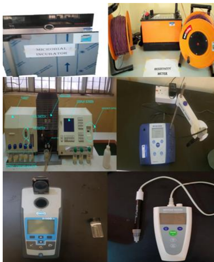
Figure 4: Microbial Incubator, Resistivity meter, Atomic Absorption Spectrophotometer and Ph meter used in the wastewater Laboratory
