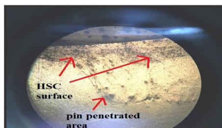
Figure 19. Shows 5X magnified c/s of the HSC coupon showing penetrated pin area.
