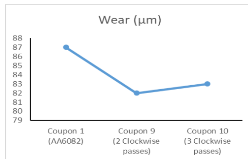
Figure 18. Shows comparison of wear between coupons 1,9 and 10.
