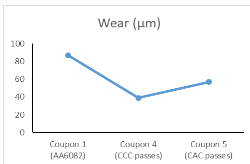
Figure 14. Shows comparison of wear between coupons 1, 4 and 5.
