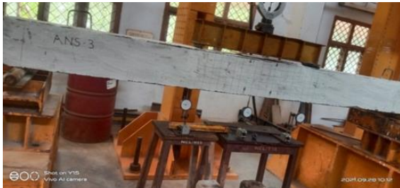
Fig. 7. Crack Patterns of Tested Beams
