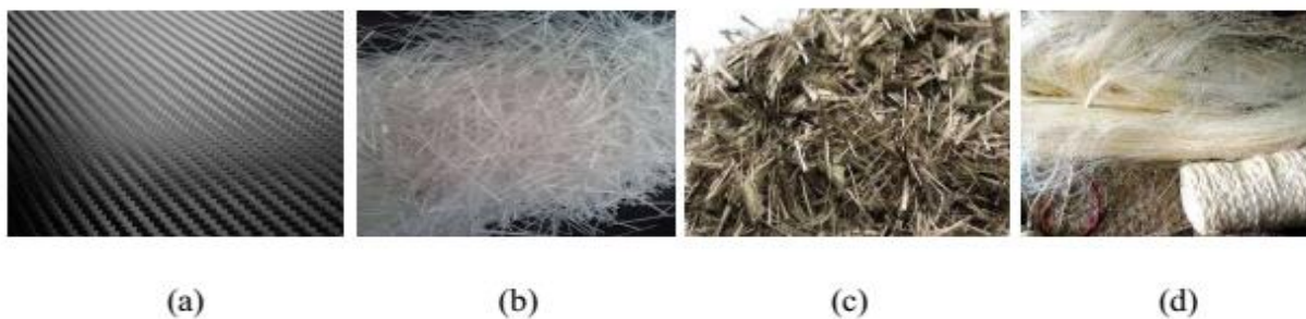
Fig 5: Fiber Materials (a) Carbon, (b) Glass, (c) Basalt and (d) Sisal
