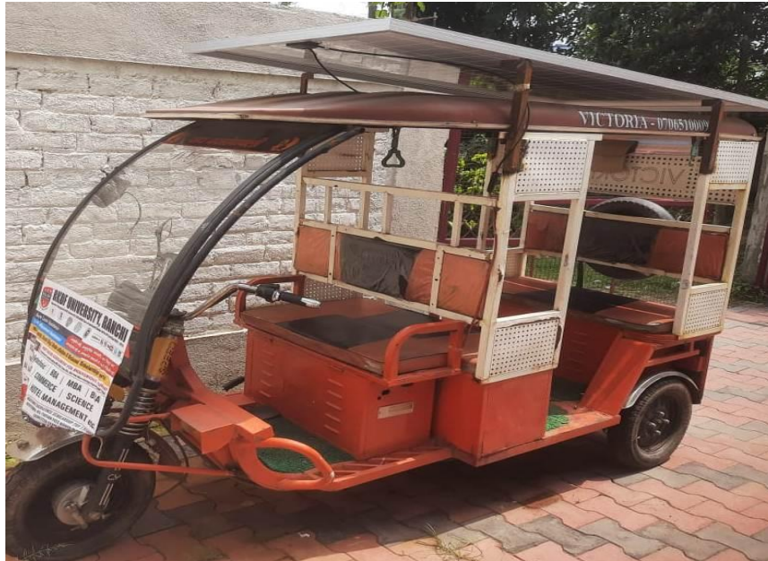
Fig 1.2: Designed and implemented Solar E-Rickshaw
