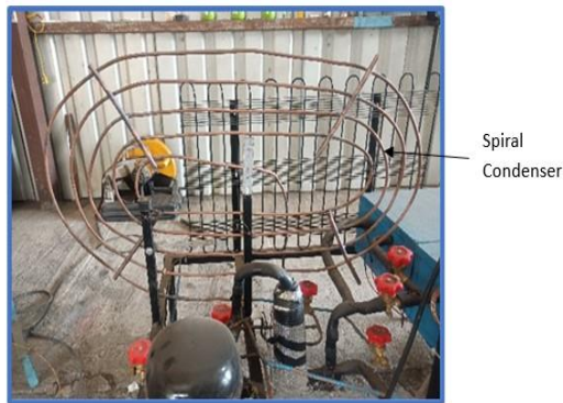
Figure 1 Spiral Condenser Arrangement
