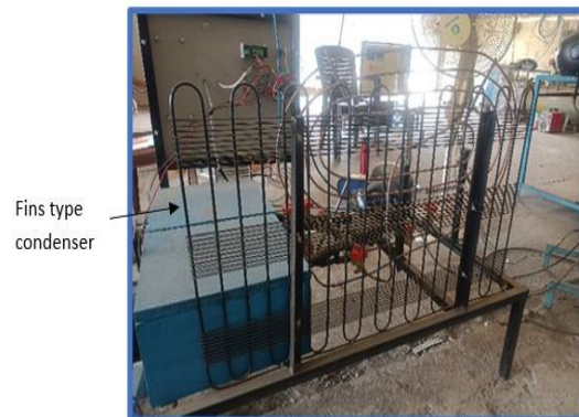
Figure 2 Fins type condenser arrangement
