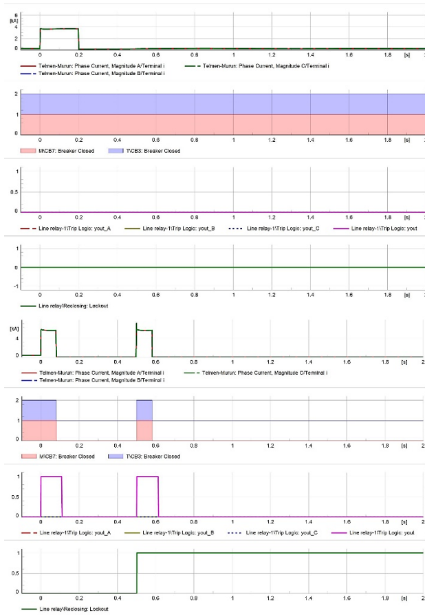
Figure 4. Model simulation result of ARC operation /3 phase short circuit successful and unsuccessful/
