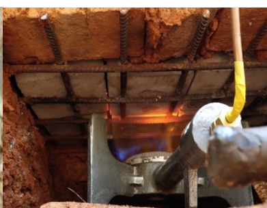
Fig. 3- Exposure of fire on concrete cubes
