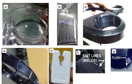
Figure 2. Common Defects Occurring during the Injection Moulding Operation
