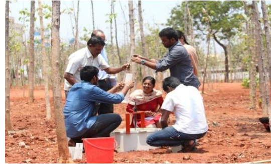
Figure 4: Water filling of lysimeter.
