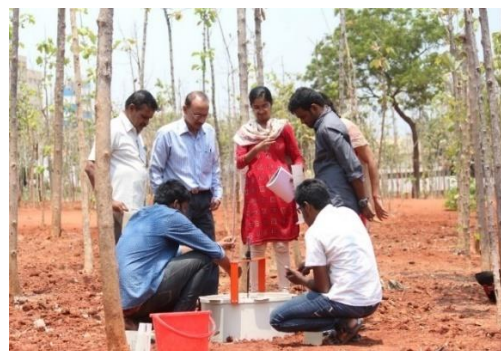
Figure 2: Lifting of filled lysimeter.
