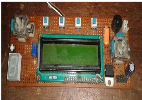
Fig 3.8 Drive-by-wire remote control
