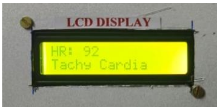
Figure 5 (b) Shows the abnormal condition condition of the heart with Heart beat 92 displayed as tachycardia.
