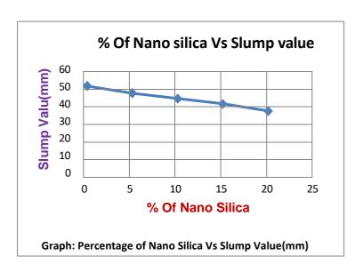
VARIATION OF SLUMP VALUE AT DIFFERENT PERCENTAGE OF NANO SILICA: From the above test results, it is observed that the Slump Value decreases as percentage of Nano silica replacing cement increases. However, the Workability is decreased with increase in percentage of Nano silica from 0%to20% of partial replacement of cement by weight.
