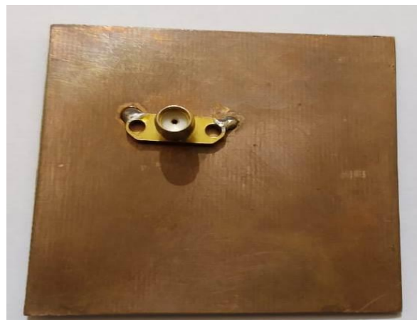
Fig.15 Probe feed point with SMA connector
