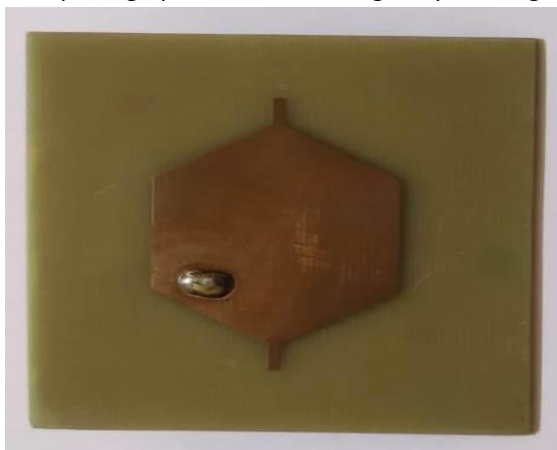
Fig.14 Top view of Fabricated Single Layer Hexagonal Stub MSA
