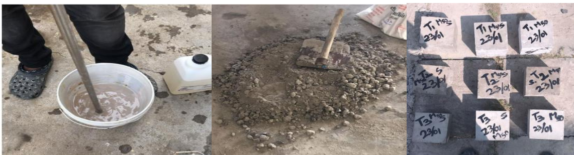
Fig.2.Preparation of Alkaline Activator Fig.3.Preparation of GPC Mix Fig.4.Ambient curing
