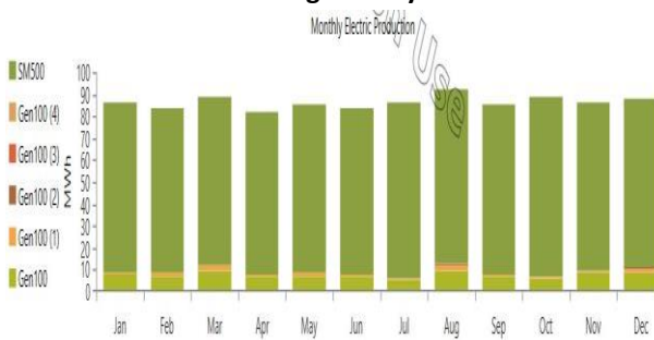
Fig.26. Monthly Electric Production for Commercial Load fed with Five 100 KW Diesel Generators and PV Integrated System
