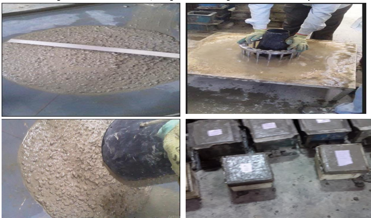
Fig.1 Free flow measurement, J-ring test and casting cubes in the laboratory
