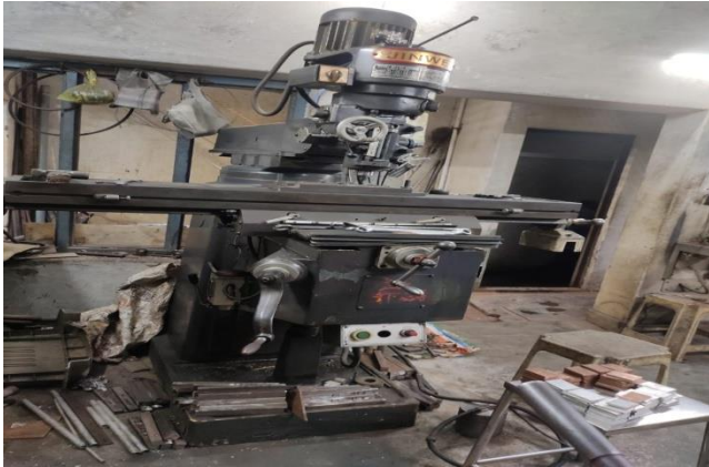
Fig. 1 Vertical Milling Machine used in FSW process Welding Details
