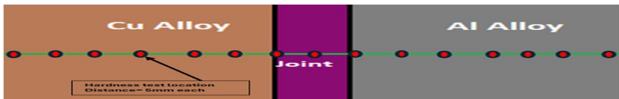
Figure 3 Hardness measurement points in Cu and Al alloys
