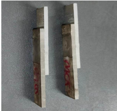
Figure 14 Figure Preparation for Tensile testing (Mg/Al)
