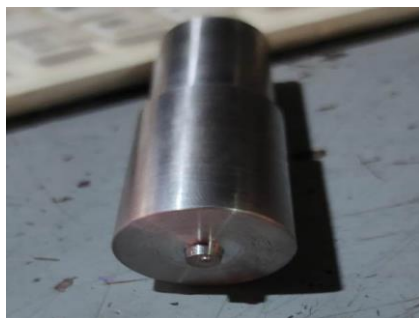
Figure 4 FSS Tool used in Experiment
