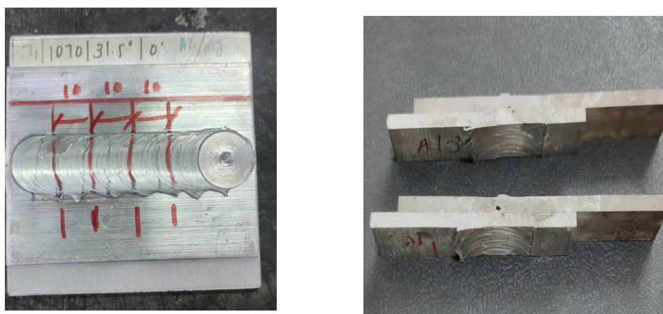
Figure 13 Preparation for Tensile testing (Al/Mg)
