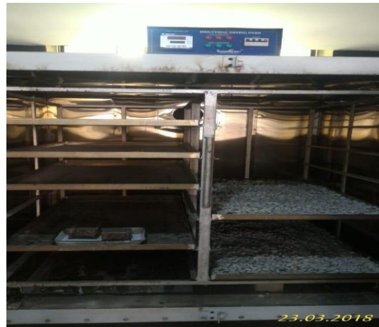
Figure: Oven curing of flyash Geopolymer Specimen
