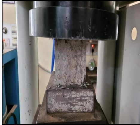
Figure: Testing for Compressive strength of concrete
