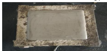
Figure: Casted flyash Geopolymer Specimen
