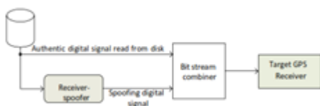
Fig 8: Spoofing test using recorded GPS data
