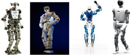
Fig.4. a) LOLA b) Valkyrie c) TORO d) RH5- Humanoid robots with the hybrid design ( Series to parallel) (Kumar, Wöhrle, de Gea Fernández, Müller, & Kirchner, 2020)
