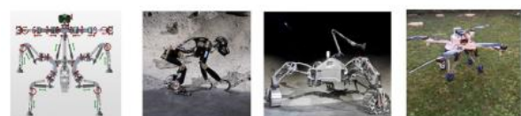
Fig. 7. A) MANTIS b) CHARLIE c) SHERPATT d) HERITAGEBOT - Hybrid design- Multi-legged robots with series-parallel.(Kumar et al., 2020)
