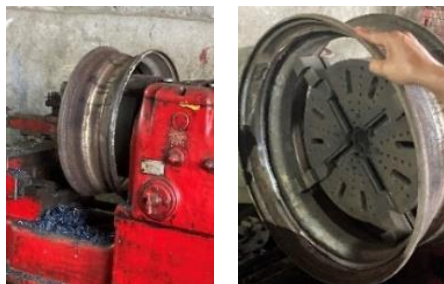
Machining after removing damaged portion
