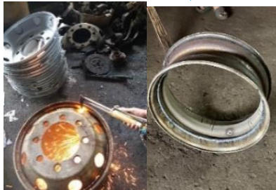
Removed damaged rim plate
