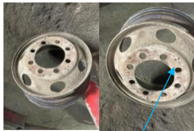
Cracked portion between holes
