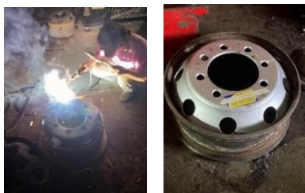
Repalced rim plate welded and machined
