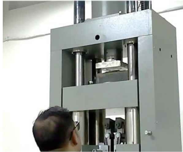
Fig.7 Compression testing of brick
