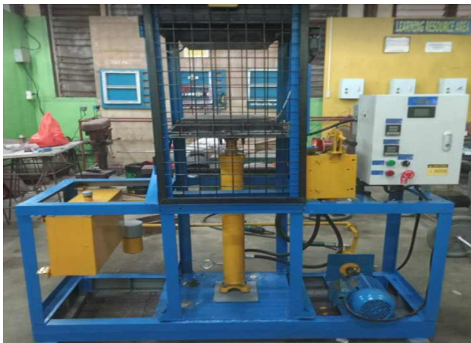
Figure 8. The fabricated hot-pressing device
