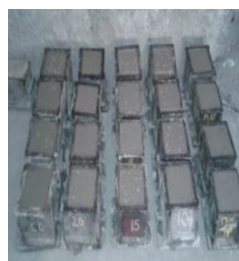
Figure 8. Cubes placed on vibrating table under compaction
