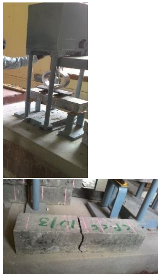
Figure 13. Flexural test on prism
