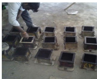
Figure 7. Preparation of moulds before casting of specimens
