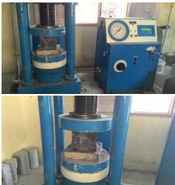
Figure 12. Compression test on cube in different view
