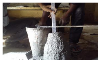
Figure 6. Slump test on first trial
