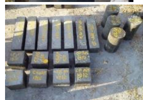
Figure10(a). Demoulded specimens after 24 hrs
