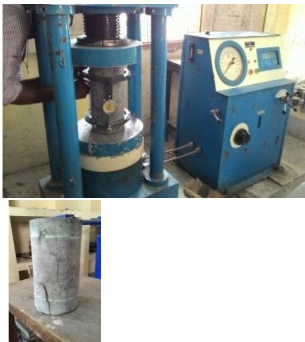
Figure 14. Compression test on cylinder
