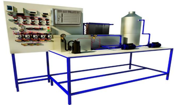
Figure 2. Perspective View of the Chilled Water Industrial Air-Conditioning System Simulator
